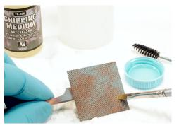
Due to the application of the Chipping Medium, the top layer of Blue 71.008 dries more slowly and can be easily scratched or peeled and flaked off with a tooth pick or other sharp object.
